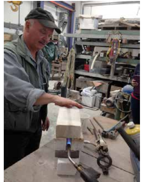
▲ AL MANGOLD DEMONSTRATES HIS SIMPLE AND INEXPENSIVE CHISEL FORGE
