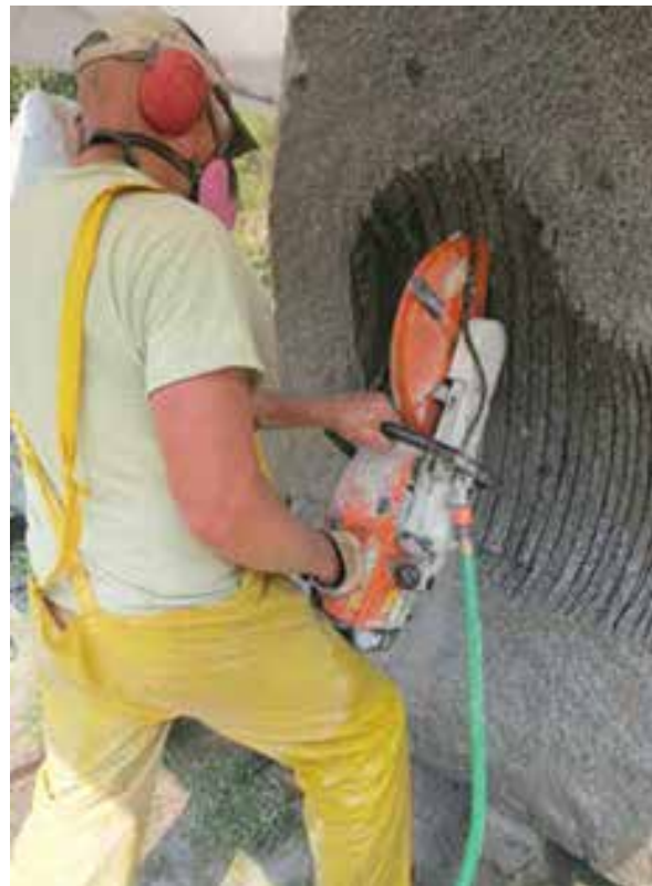
▲ BOB USING A GAS-POWERED 14" CUT-SAW WITH A WATER FEED TO ROUGH OUT THE BOULDER SCOOP-OUTS.
