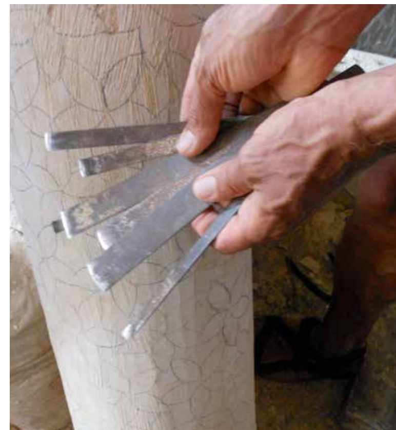
▲ SOME OF THE SIMPLE STONE CARVING CHISELS USED IN BALI
